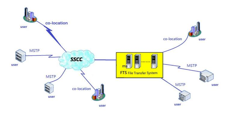
Figure 2-1 FTS User Access Network Diagram
