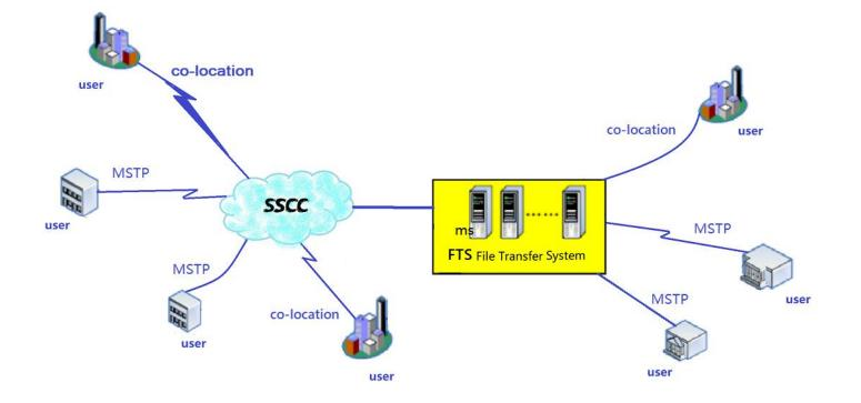
Figure 2-1 FTS User Access Network Diagram
